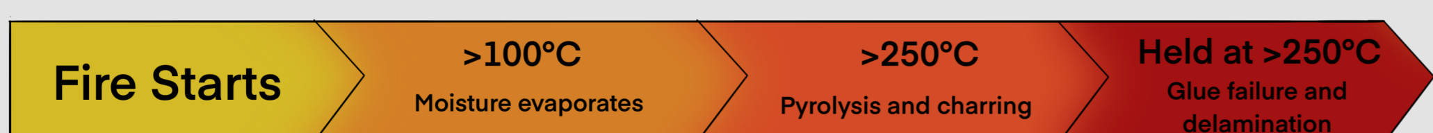
Above: Timeline of the behaviour of laminated timber when exposed to fire.
