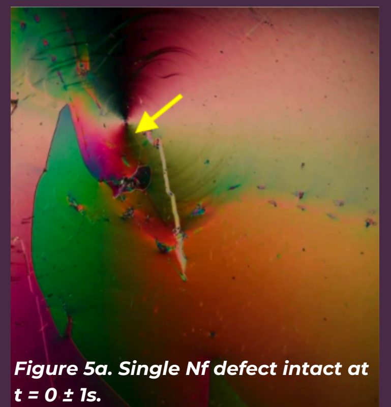
Figure 5. An induced electric field causing the characteristic N_f defect line to split at the sub-transition temperature of 43 \pm 0.1^\circ\text{C} .
