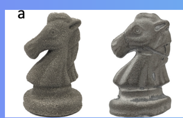
Figure 3 CIPed and FASTed part [3]
