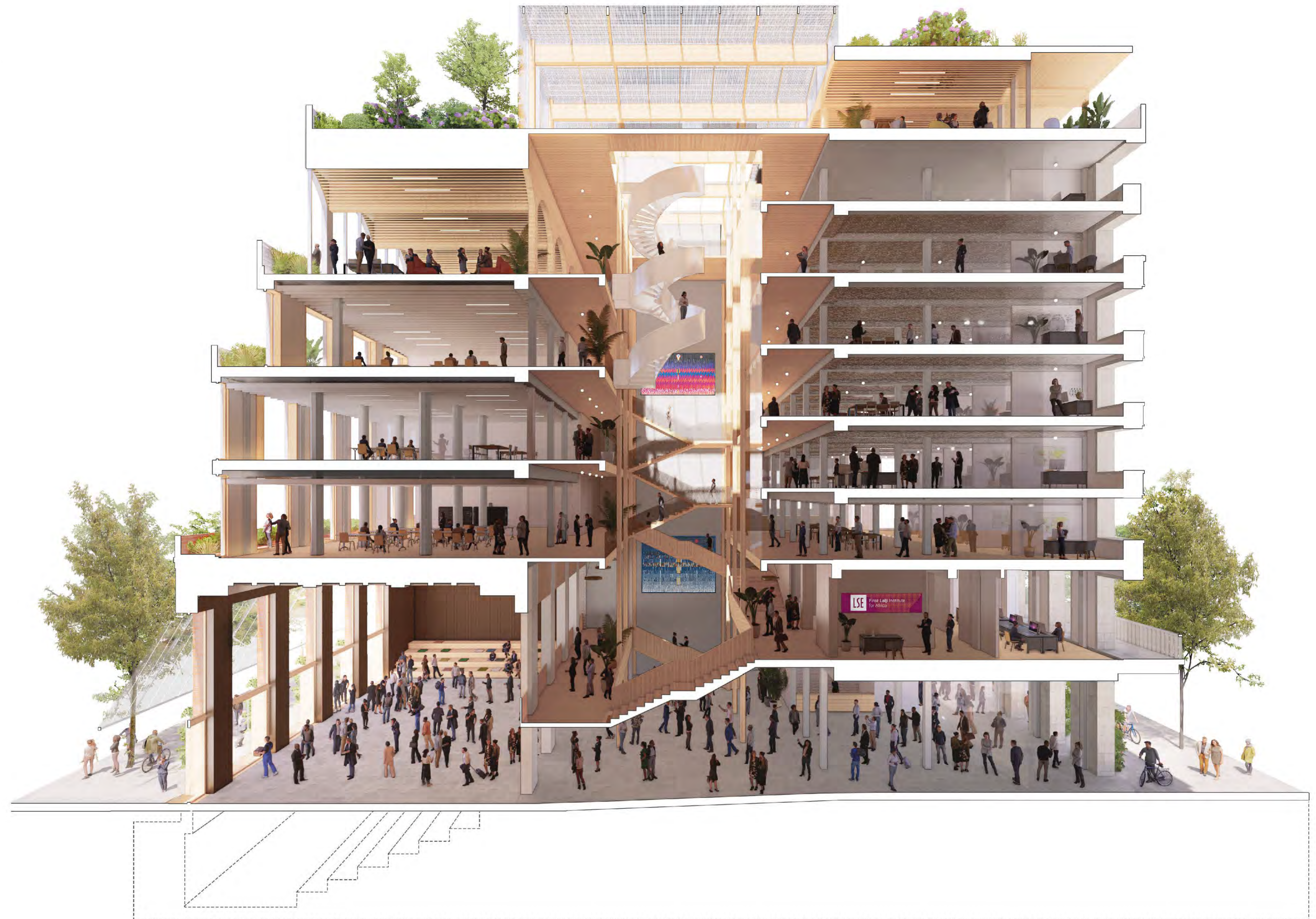
Cross section showing the diversity of spaces throughout the building which open to both LIF and Portugal Street. A central atrium, which also serves as exhibition space, provides a dynamic area and draws daylight through the building.
