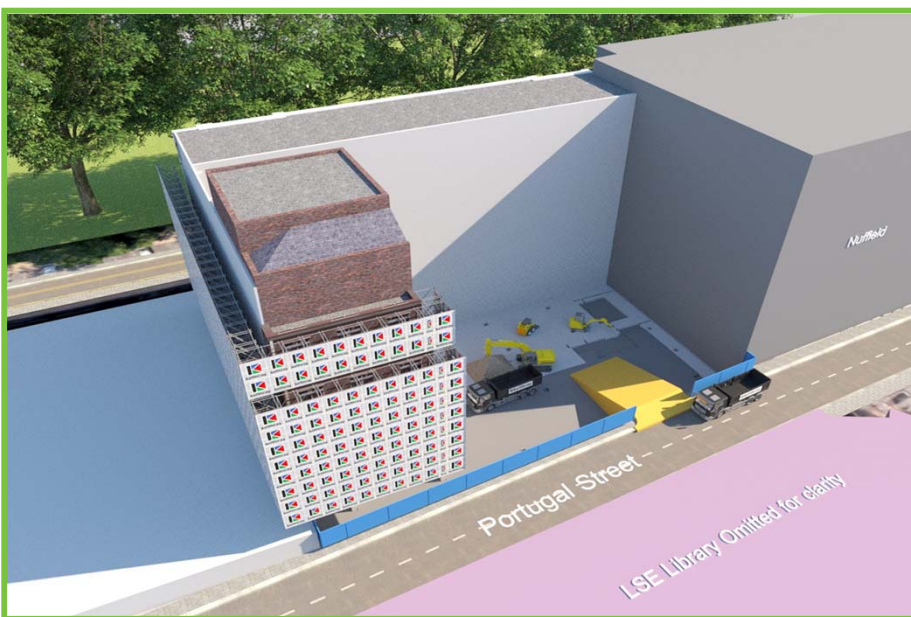
Fig 06 - Synchro Image of demolition from Portugal street
