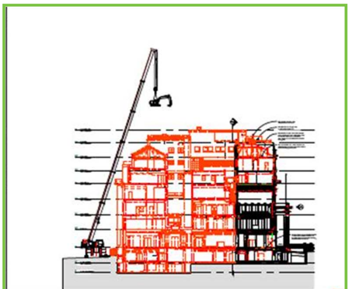
Fig 08 - Position of mobile crane on Portugal Street
